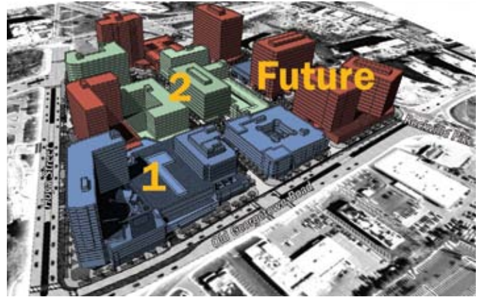
The phasing plan for the Pike and Rose project shows how density will be incrementally added by increasing height and constructing new streets. (FEDERAL REALTY INVESTMENT TRUST)
